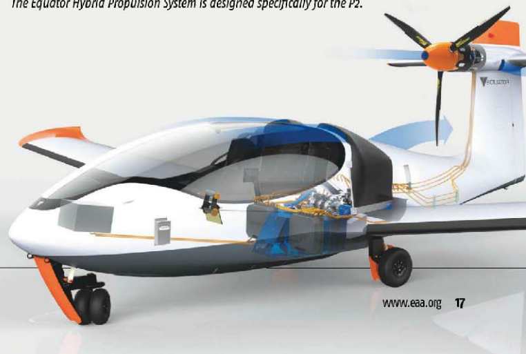
The Equator Hybrid Propulsion System is designed specifically for the P2.
